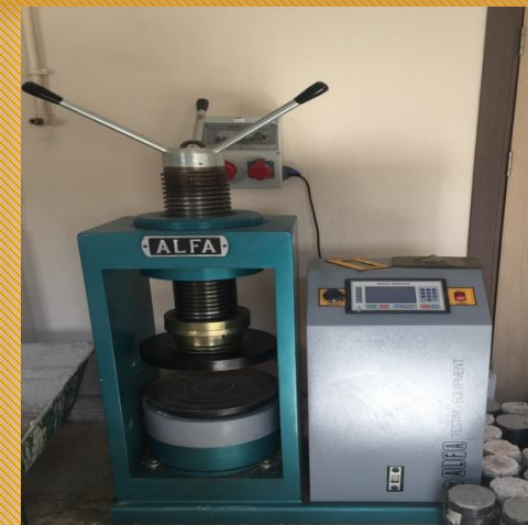
Concrete Compression Testing Machine
