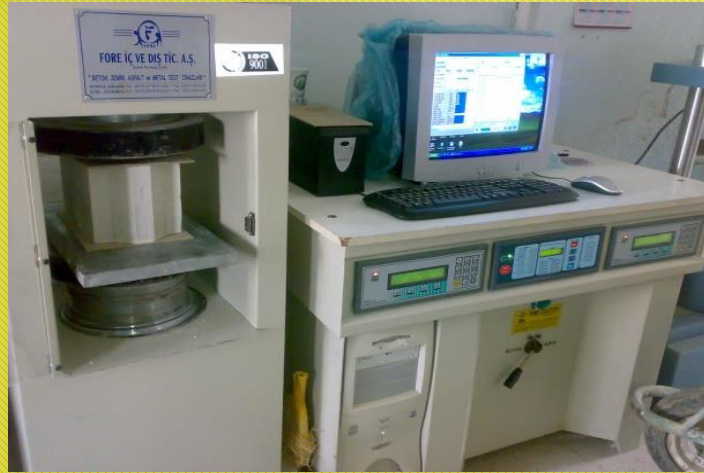
Concrete Compression Testing (200 Tons) and Flexure Testing (20 Tons) Machine
